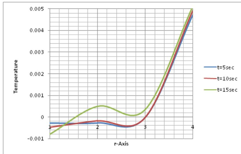
Fig. 3. Transient temperature variation in the radial direction at different time
