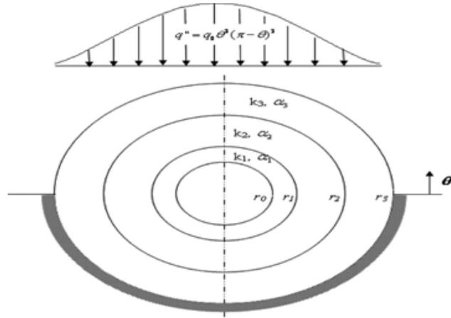
Fig. 2. Discretized model of multilayer circular annulus
