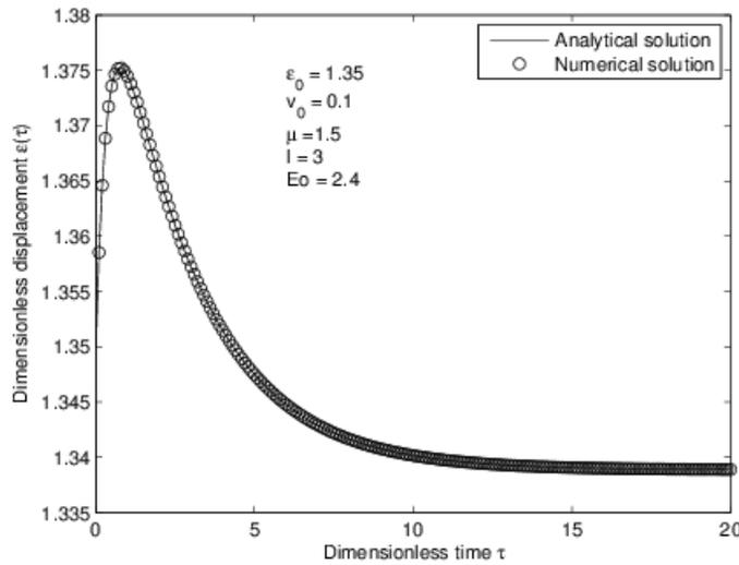
**Fig. 1.** Comparison between analytical (solid line) and numerical (circles) solutions for viscously over-damped nonlinear forced response
