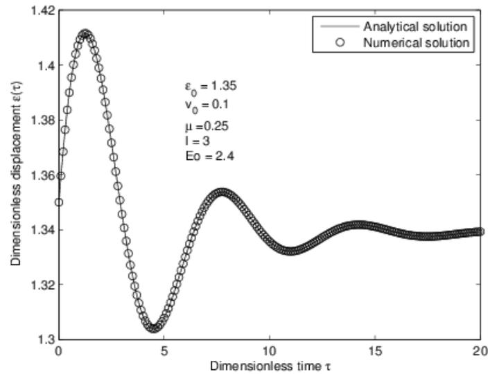
**Fig. 5.** Comparison between analytical (solid line) and numerical (circles) solutions for viscously under- damped nonlinear forced response
