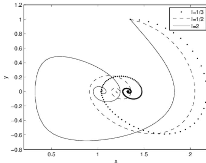
**Fig. 13.** Effect of hardening nonlinearity on the steady state deformation simulated in the phase plane
