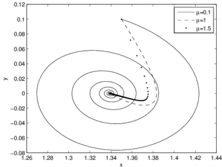
Fig. 11. Effect of viscous damping on the steady state response
