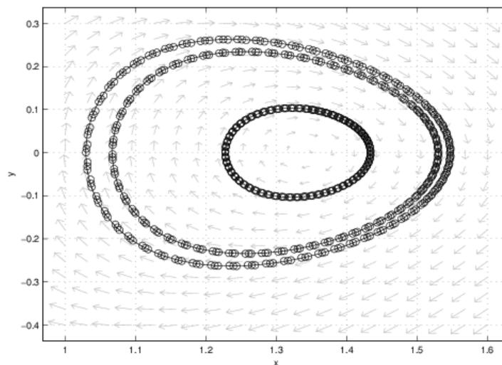
**Fig. 8.** Phase orbits of the analytical (solid line) and numerical (circles) solutions for non-viscously damped nonlinear forced response
