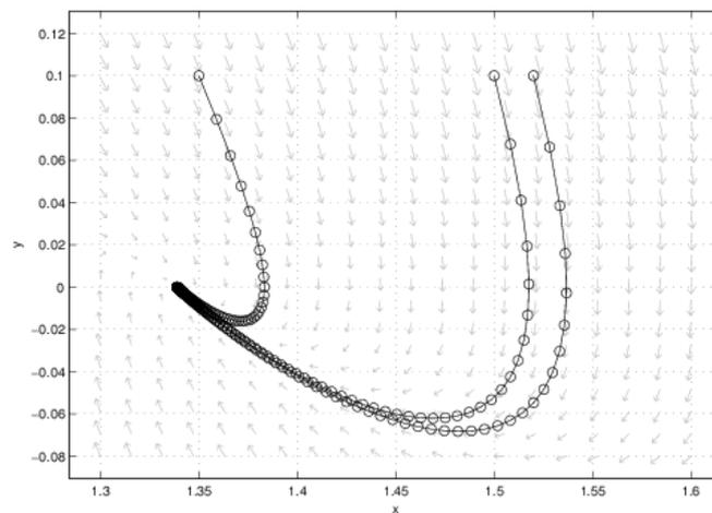
**Fig. 4.** Phase orbits of the analytical (solid line) and numerical (circles) solutions for viscously critically damped nonlinear forced response
