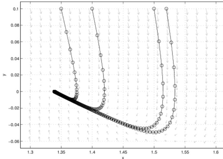
**Fig. 2.** Phase orbits of the analytical (solid line) and numerical (circles) solutions for viscously over-damped nonlinear forced response
