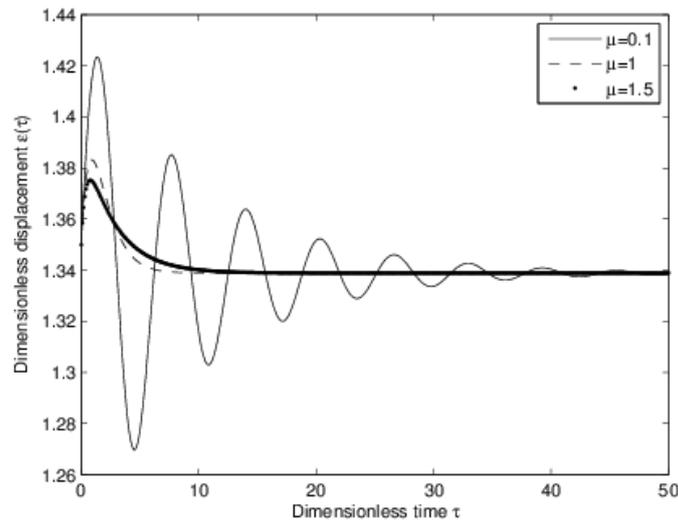
**Fig. 10.** Effect of viscous damping on the steady state response
