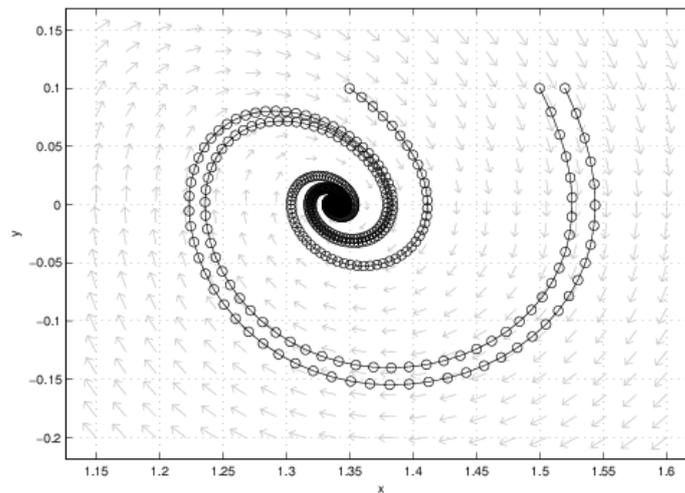
**Fig. 6.** Phase orbits of the analytical (solid line) and numerical (circles) solutions for viscously under-damped nonlinear forced response
