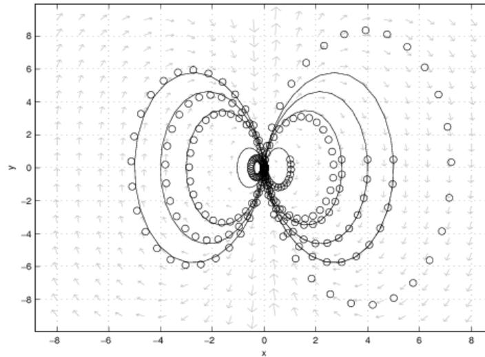
**Fig. 9.** Phase orbits of the analytical (solid line) and numerical (circles) solutions for non-viscously damped nonlinear free vibration response
