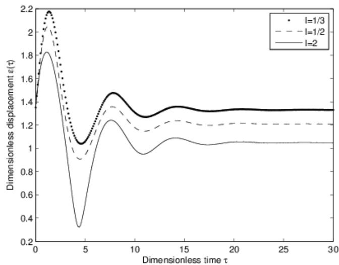
Fig. 12. Effect of hardening nonlinearity on the steady state deformation
