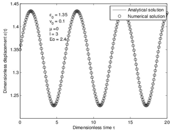
**Fig. 7.** Comparison between analytical (solid line) and numerical (circles) solutions for non-viscously damped nonlinear forced response
