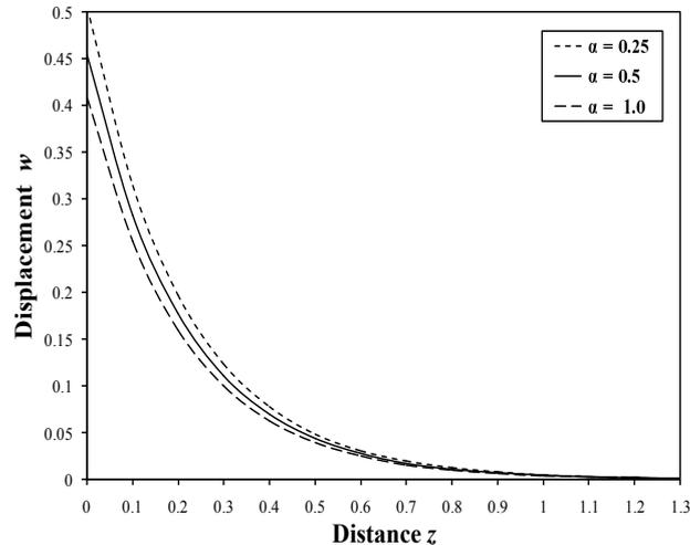
Fig. 1. Effect of fractional parameter  $\alpha$  on the distribution of displacement  $w$  at  $t = 0.1$
