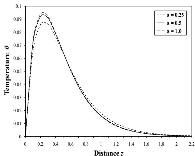
Fig. 2. Effect of fractional parameter  $\alpha$  on the distribution of temperature  $\theta$  at  $t = 0.1$
