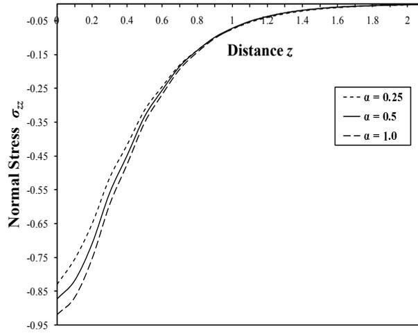
Fig. 3. Effect of fractional parameter  $\alpha$  on the distribution of normal stress  $\sigma_{zz}$  at  $t = 0.1$
