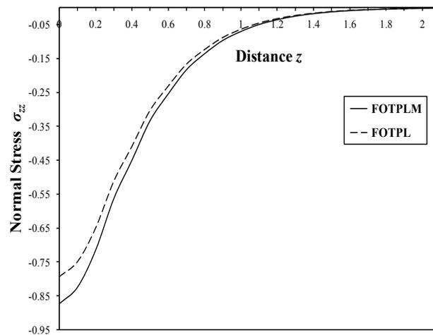
**Fig. 6.** Effect of magnetic field on the distribution of normal stress  $\sigma_{zz}$  at  $t = 0.1$  and  $\alpha = 0.5$
